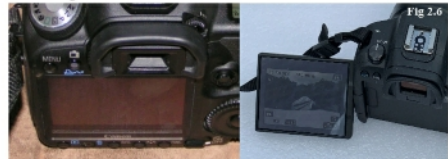
Canon C50D DSLR Fixed LCD display (left) and R6 Mirrorless tilt-able display (right)
